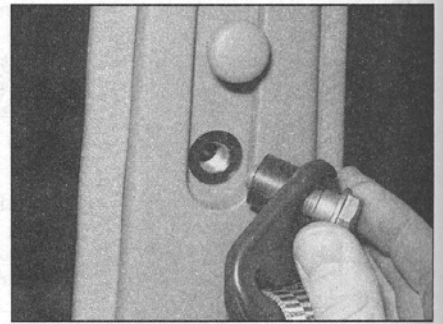
25.1b . . . then undo the retaining bolt, and recover the spacer which is fitted between the seat belt and pillar
