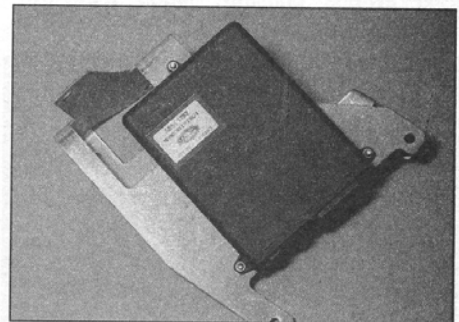
18.11 Window lift control unit is secured to its bracket by three nuts
