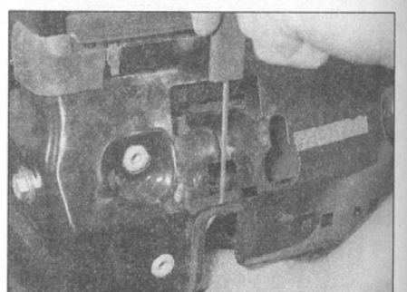
13.14 Release the retaining clip, and detach the lock button from the lock
