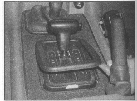
27.6 Unclip and remove the selector panel surround
