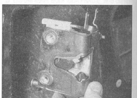
13.17b . . . and withdraw the lock assembly from the door
