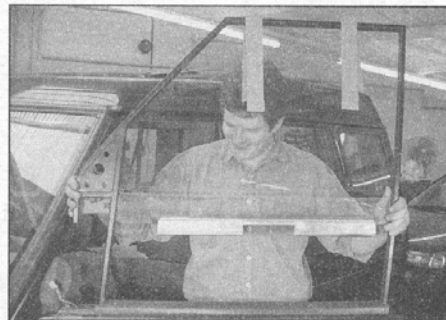
14.9 ... then lift the frame and window glass assembly out from the door
