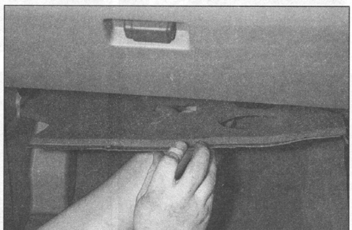
28.16b . . . and remove the lower covers from the fascia
