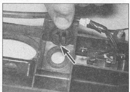
16.22b ... and recover its O-ring from the number plate housing
