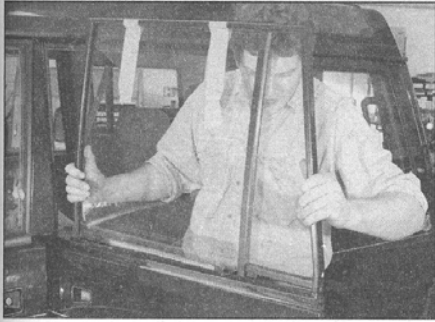
14.15 ... then lift the window glass and frame out from the rear door
