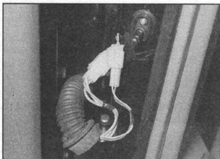
11.8b ... and withdraw the rear door wiring connectors from the pillar
