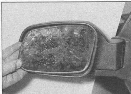
19.11 Remove the mirror glass as described in text ...
